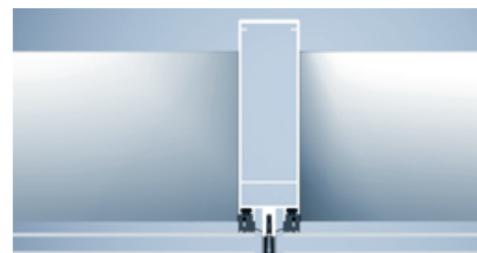
integration profile with sun protection bolts
