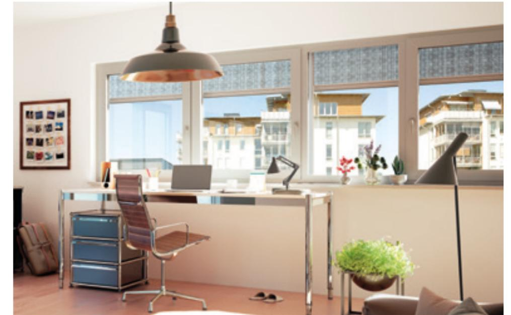
This textile sun protection is installed outside, in front of the window. Depending on the fabric chosen, the sun protection can be either transparent or non-transparent. The textile reflects and absorbs sunlight, thereby reducing sun radiation by up to 100 %. That means you do not have to go without natural daylight. At the same time, UV-radiation is filtered by up to 100 %.
